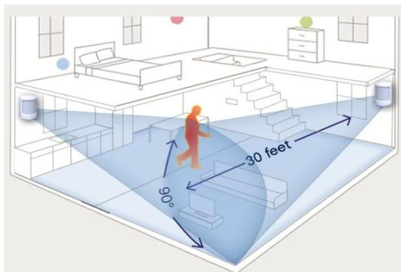
Fig.4. Use of Motion Sensor
