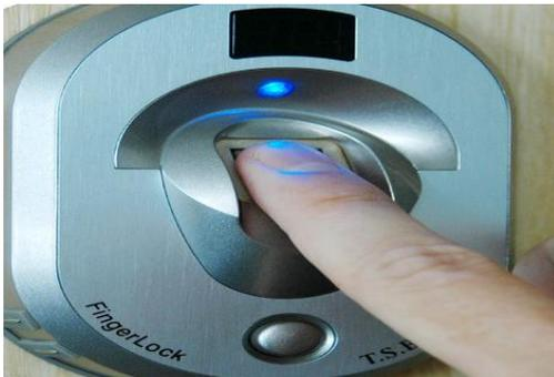
Fig.7. Fingerprint scan
